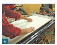
Remove the base and drill about four pilot holes down the length of the runner, counter sink and secure in place with screws.
