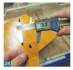
Then cut a 30mm piece off side 5 – label the top A and bottom B. Any angle error between the blade and fence has now been compounde four times.
