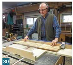
29 Now cut a piece of wood on the sled, measuring should confirm that the sled is now ready to make accurate, repeatable 90° cuts.
