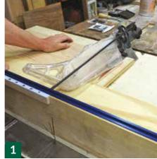
cut to size. I used a cheap piece of 19mm ply as it was unlikely to be seen. **Note:** when cutting mitres, it is always safer to use a sled. Never try to do this against the fence.
