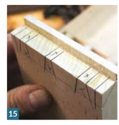
16 Saw on the waste side of the line and chop out the waste using the method described above. When cutting tails, it's sometimes easier to angle the wood so that the saw is cutting vertically.
