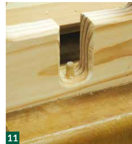
7 The template for the centrepiece of the puzzle, which will need to be a good fit.
