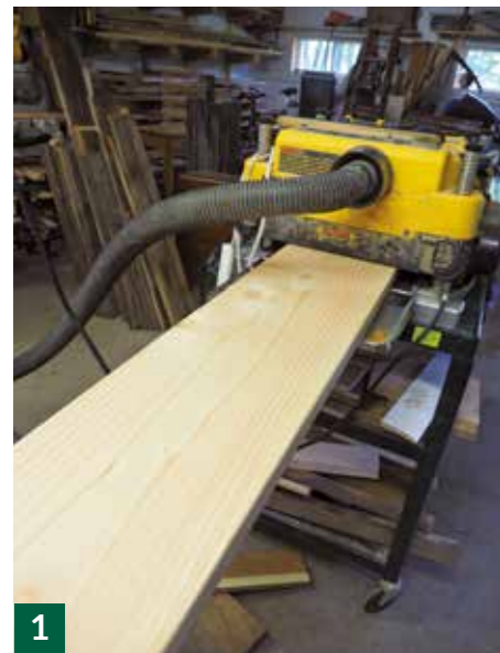
1 First the pine boards were run down to 32mm final thickness.
