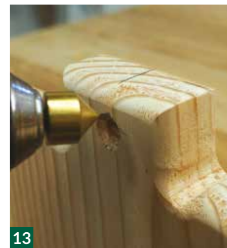
13 Note the scoop out at the foot of the tenon, which helps it all fit together easily.
