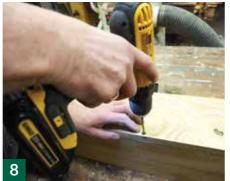
I only had enough dowelling for seven supports!). However, you decide on the positioning, adjust the spacing and quantity of supports accordingly. Drill the holes (slightly under-sized).
