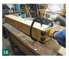
wood in. Place a bucket under the drain holes. If you make this out of pine, the smell and the sap steaming away is quite aromatic. As a guide, it takes about 1 hour of steaming at 215°F for every 25mm of thickness, but wood will vary with species.
