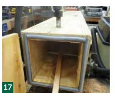
**1** Secure a 25 x 25 x 180mm block of wood about 50mm from the front of the box.
