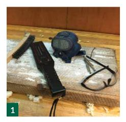
foreign material. Where I live it is not uncommon to find nails, barbed wire and even the occasional bullet embedded in the wood. I suggest using a metal detector, wire brush, facemask and eye protection when cleaning old wood.
