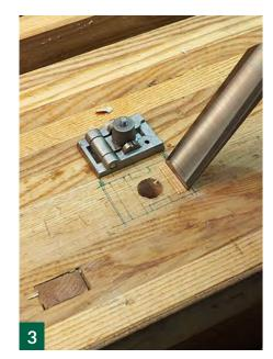
• With a wide chisel, start to chop out • The mortise. Make sure to go easy because one side of the dog is about half the depth of the other.
