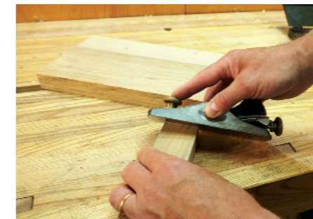
Easing the edges and adding a chamfer
