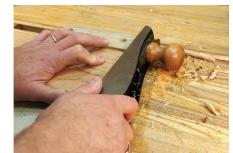
Using the bench hook for shooting ends
