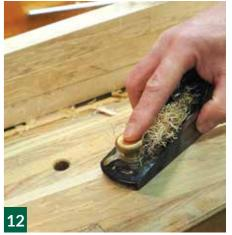
a jointer plane. Be careful not to encroach beyond the upper marks as it will ruin the mating surface between the rail and the leg.
