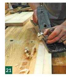
21 Plane mating pieces together; this way the joint is pretty much guaranteed to fit. This technique was explained in detail in my project on making a table top in *Woodworking Crafts* issue 2.
