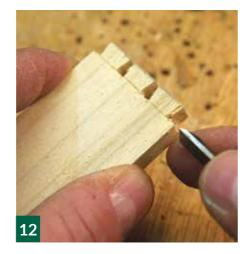
line and held close to the end for control, chop half way through the wood. Turn the pieces around and repeat from the other side. Finally, place the chisel in the knife line and chop out the last bit of waste. I always do this last chop from the face side so that if there is any tear-out, it will be hidden inside. Clean up the tails.
