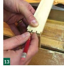
in the vice with the face towards you, place one of the sides on top so that the knife line matches with the ends of the tail. With a very sharp knife or pencil, draw it towards you along each tail edge. Do not draw the knife past the knife line on the end grain.
