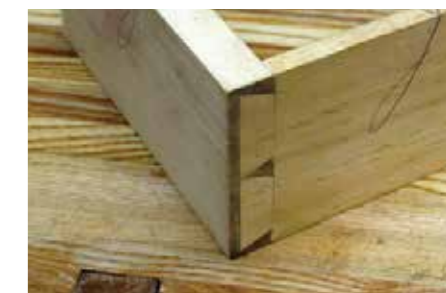
Lapped dovetail or half-blind dovetail
