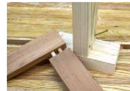
Stud joined with nails or screws and a dowel joint, both examples of using mechanical means to joint end grain to long grain
