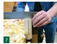
7 However, this is not an excuse for abandoning square edges. Check with a try square at discrete intervals along the length; a back light will help to see where you need to plane more; mark these areas with a pencil and plane the marks off.
