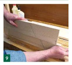
a few passes with the Jack plane to bring the roughness down. With this step we are not trying to smooth the surface completely and visible plane marks are quite acceptable and add to the finished hand tool look.
