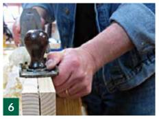
Take adjacent boards and place O the sawn faces together and clamp them in the vice. Planing two boards in this manner serves two purposes: a) it provides a more stable surface to plane on; b) while ideally we want to plane perpendicular to the faces, errors do occur and any angle introduced into the planed surface will be compensated for in the other piece.
