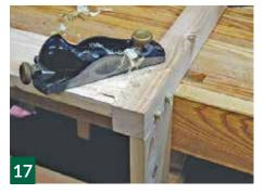
to split out any fibres. It's a good idea to 'ease' the end-grain from both sides first. While you are at it, clean up all the legs and skirt with the block plane.
