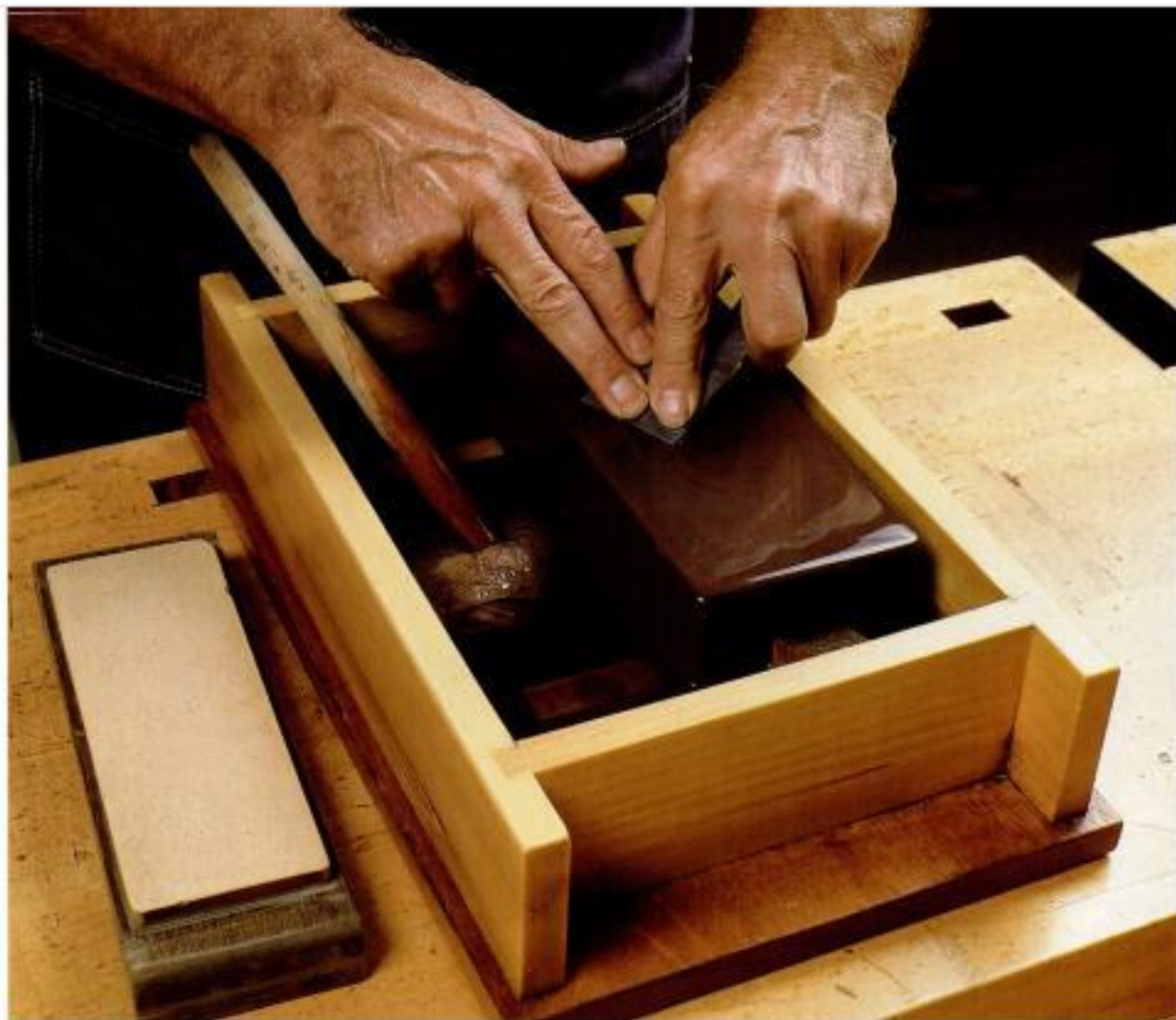
Watertight container. Klausz's wooden box keeps his waterstone wet for sharpening.
