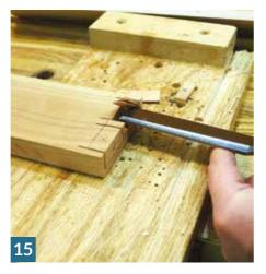
Z Test fit the joints. With dovetails 16 it is important to not over-test as this makes for a sloppy fit. If you do need to tweak the fit, go easy. As these are custom-fit dovetails it's a good idea to mark the mating boards. The extra 1mm that was added in the beginning can now be planed off.
