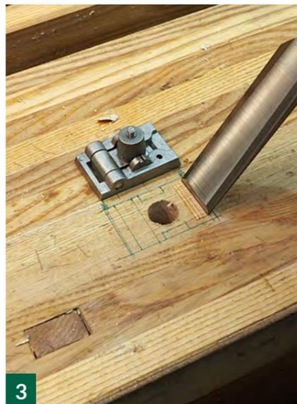
**3** With a wide chisel, start to chop out the mortise. Make sure to go easy because one side of the dog is about half the depth of the other.
