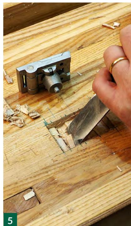
**5** Work the section that will house the hinge. With the bevel down, make pivoting cuts from both sides.
