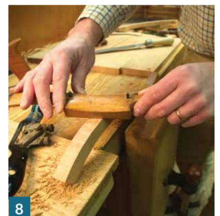
**Cutting the sliding dovetail**
